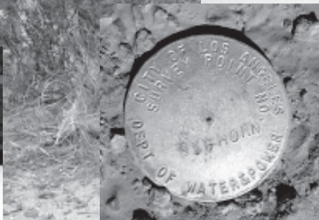
An LADWP survey marker, cemented into the ground (left). Similar survey markers, accompanied by marking stakes, have been found in half a dozen locations on BLM and private lands.
